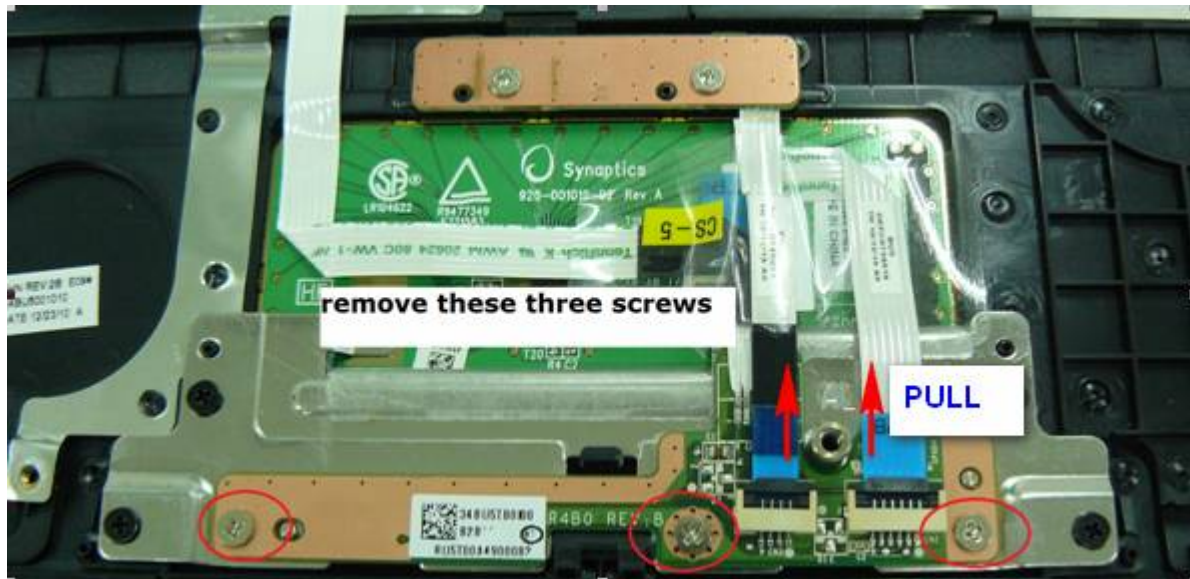
Figure 4-7-2 Remove the touch pad board
