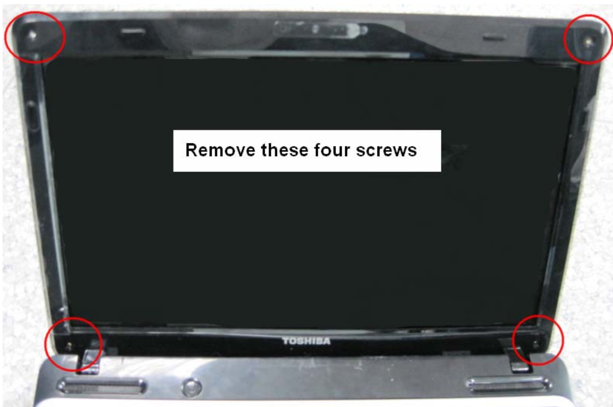
Figure 4-13-1 Remove the display mask
