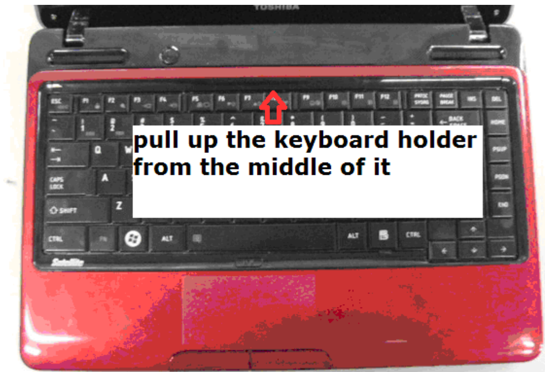
Figure 4-3-1 Remove keyboard holder
